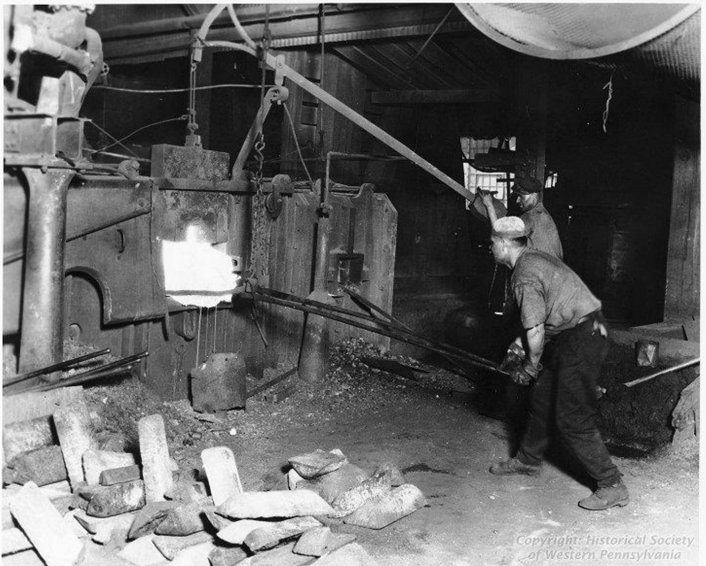
Puddlers remove an iron ball from a puddling furnace
